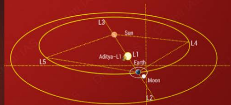
Illustration of all five Lagrange points of Sun-Earth System. Aditya-L1 will be placed around Lagrange point 1
